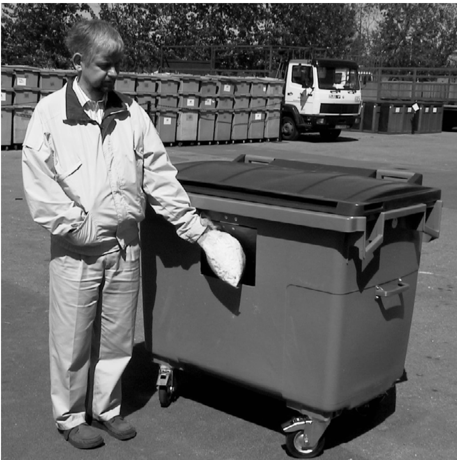
Figure 10. The 600 litres 4-wheeled bin was equipped with a top-hinged, 30 x 30cm inlet fitted at the receptacle's front as a supplement to the lid. The cut-out piece was used as an inlet: when pushed forward the bin bag is deposited in the waste bin. The height of the inlet, measured from the lower limit of the aperture to the ground level, was 70cm. The modified waste bin was equipped with wheel-locks.
