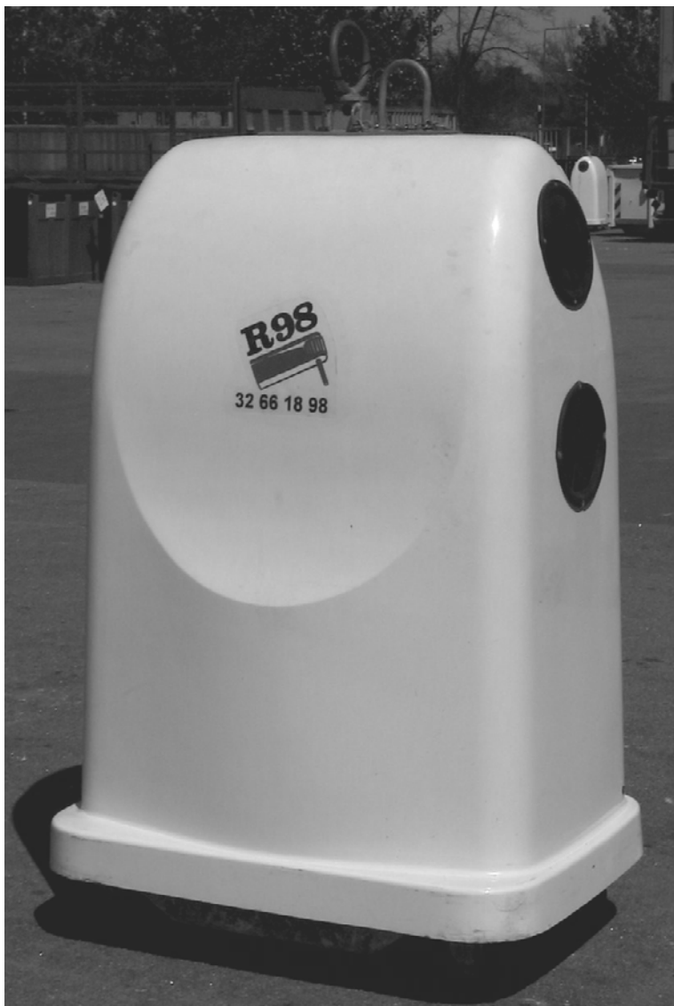
Figure 13. The 900 litres glass bank was fitted with two circular inlets, placed at different heights. The height of the lower inlet, measured from the lower limit of the aperture to the ground level, was 85cm. As standard equipment, the glass bank was fitted with wheel-locks.
